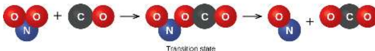
Figure 12.17 The probable mechanism for the reaction between \text{NO}_2 and \text{CO} to yield \text{NO} and \text{CO}_2 .
