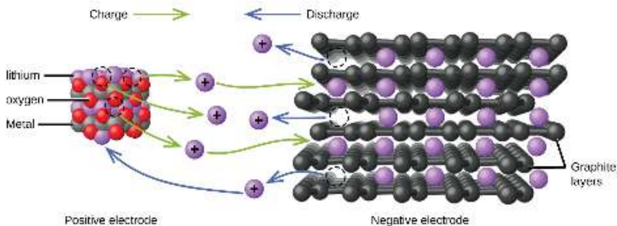
Figure 17.12 In a lithium ion battery, charge flows as the lithium ions are transferred between the anode and cathode.
